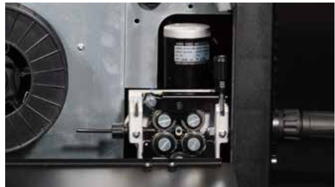
Wire Feeding system of PROMIG 200SYN PULSE
